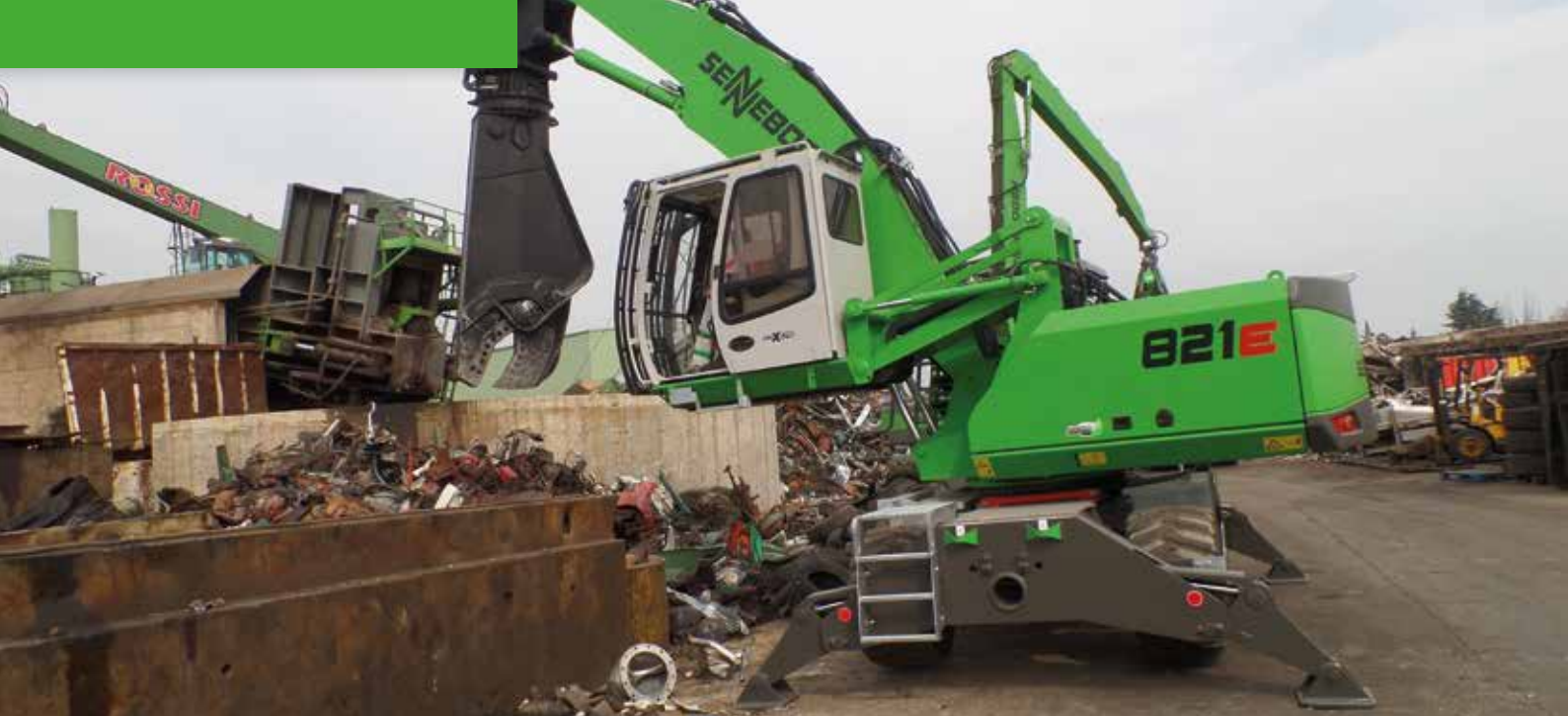
Schrottschere statt Stiel Scrap shear instead of stick
